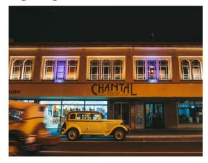
Lighting should be considered early in the design process and be integrated with building design. Spotlights or small floodlights can be used to accentuate building features such as plasterwork, niches or a balcony.
