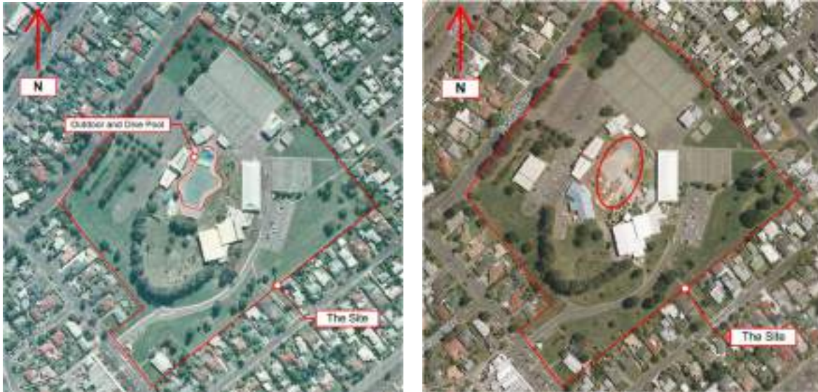
Figure 2.1: Aerial photograph from 1999 (left) showing position of outdoor swimming and diving pool and aerial photograph from 2015 (right) showing this remove and backfilled.
